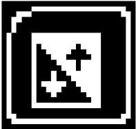
Contrast Icon – Select this to adjust the display contrast. Use the up and down arrows to adjust and press OK to save the settings
